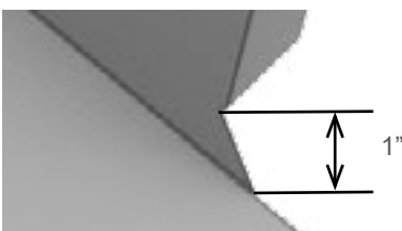
Closeup of 1" Water Diverter
